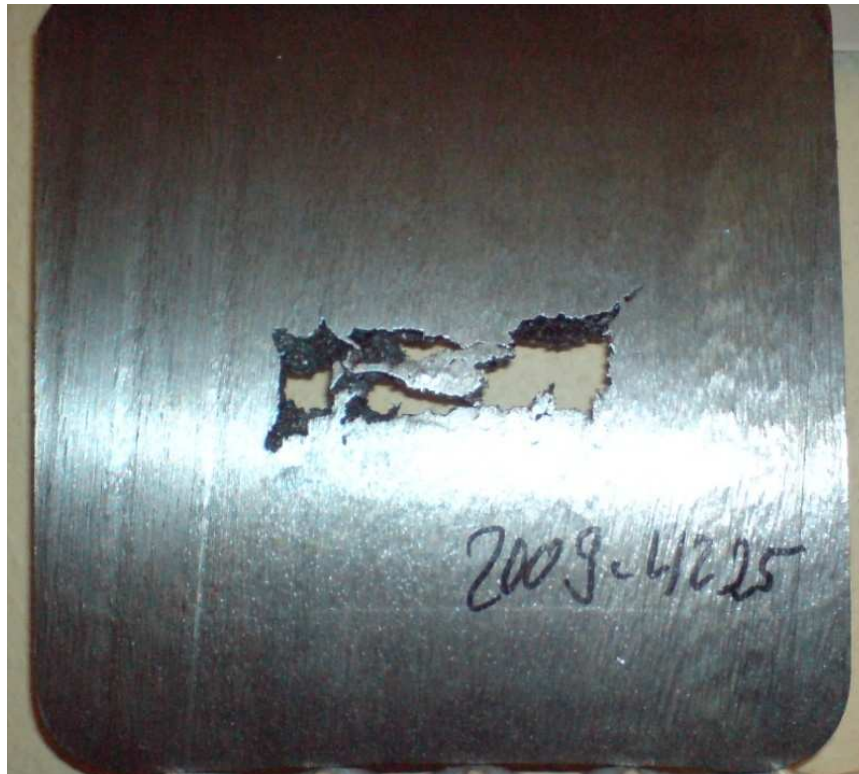
großer Lunker in Blockmitte
